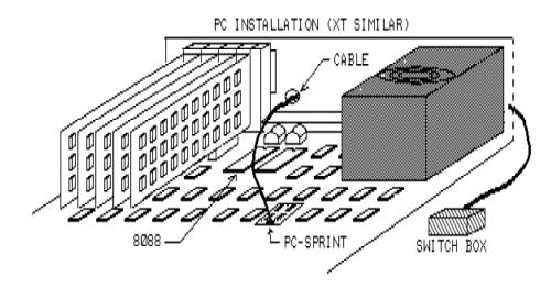
First, and most important, unplug the computers power cord from the outlet to prevent any possibliity of shock. While you're at it, disconnect all external cables (crt, keyboard, printers, modem, etc.) to protect them from you and you from their power systems.
