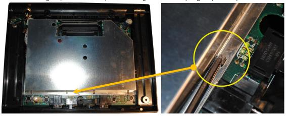
3. Locate the area where wires will be attached on the resistor ladder section just to the right and below the RF modulator area. The area circled in yellow is the resistor section for video taps.
