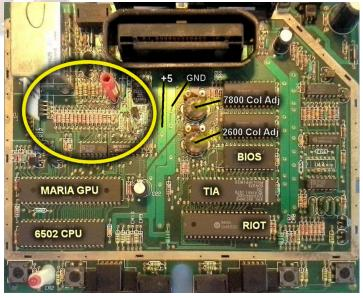
9. Solder the other ends of your resistor connection wires from the UAV to the following locations on the South legs of the resistors shown below. **NOTE: 1 on the UAV matches to 1 on the resistor labels below. So 1 to 1, 2 to 2 and so on. Trim your wires as needed for proper length.**
