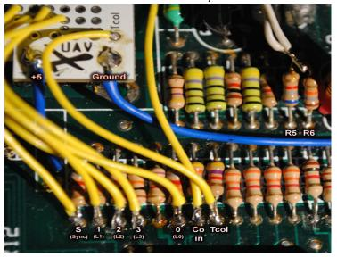
12. Cut the North legs of these two resistors and solder the ends together. Solder the '+' leg of a 10uf/16v capacitor off the North leg connections or attach using a length of wire if that is easier. The '-' leg of the capacitor will attach to the centers of your audio out RCA jacks.
