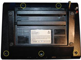
2. Remove the upper RF shield by using your needle nose pliers to twist the hold down metal tabs and make them stand straight up and flat so they will fit through the slots they originally come up from.
