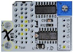
7. Solder your wires from the UAV Video out section that will be connected to your AV out connections: (Chroma & Luma are for S-Video, Comp Video is Composite)
